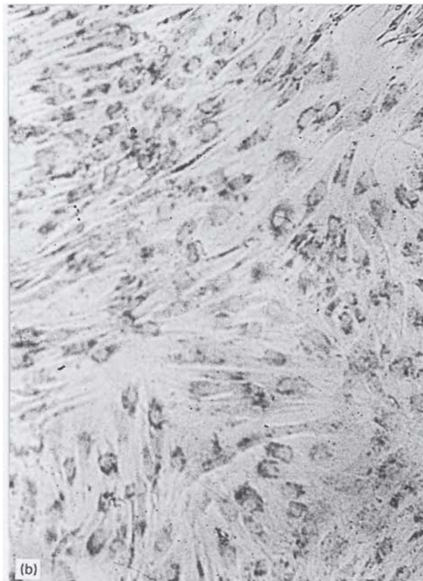
Figure 7 Mild toxic response to the extract of VS-treated HA powder: decrease of cell density (X 200): (a) control; (b) VS extract.
